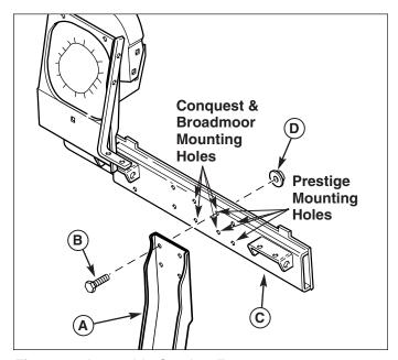
Figure 5. Assemble Catcher Frame
